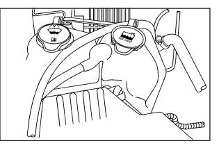
When the engine is cold, the coolant level should be at least up to the FULL COLD mark. If it is not, you may have a leak at the pressure cap or in the radiator hoses, heater hoses, radiator, water pump or somewhere else in the cooling system.
